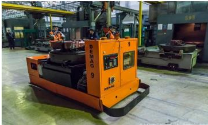
Figure 3.3.3 - Robocar (automatic cart)
