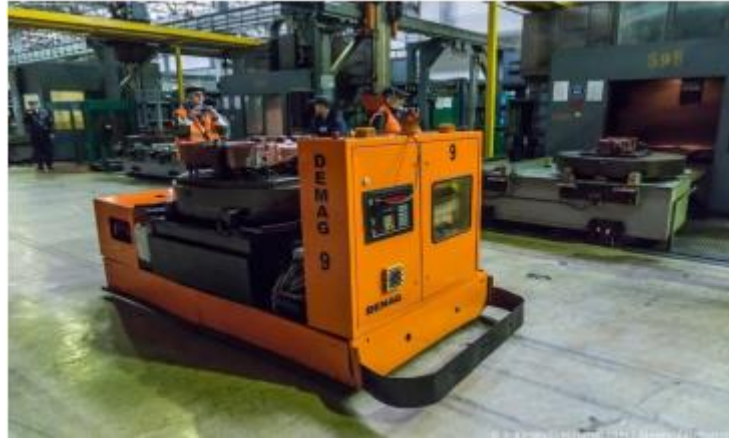
Figure 9.3 – Robocar (automatic cart)
